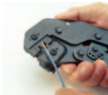
7. The result will be a perfect termination.
